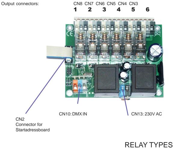
This decoder is fitted with contact relays designed for a switching current of **max 10A at 230V** (resistive load only!). When selecting and ordering the appropriate relay card, please note, that all data given by the relay manufacturers are for **RESISTIVE LOAD** only. Incandescent lamps may be considered resistive loads. Switching inductive loads, such as transformers or solenoids, requires
