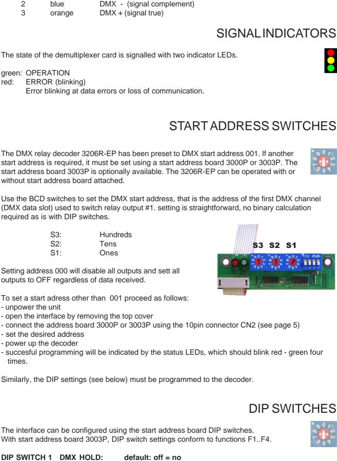
Use the BCD switches to set the DMX start address, that is the address of the first DMX channel (DMX data slot) used to switch relay output #1. setting is straightforward, no binary calculation
